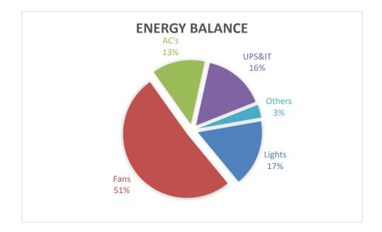
51 % of the total energy consumed in this facility is used to operate Fans. Lighting uses 17% Air-conditioners uses 13%. UPS and IT equipments Using 16%. Other equipment like pumps, Laboratory etc. uses 3%
